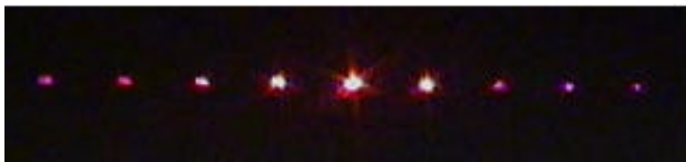
Figure 10: The diffraction pattern of a linear grating.
